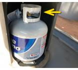
Find valve at top of tank Turn clockwise to OFF
